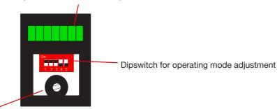
Potentiometer for adjustment of the hole size:
