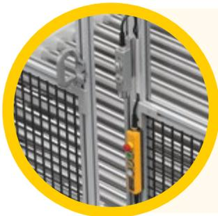
Operational unit and monitoring of the safety switch (e.g. tGard) on the sliding door.
