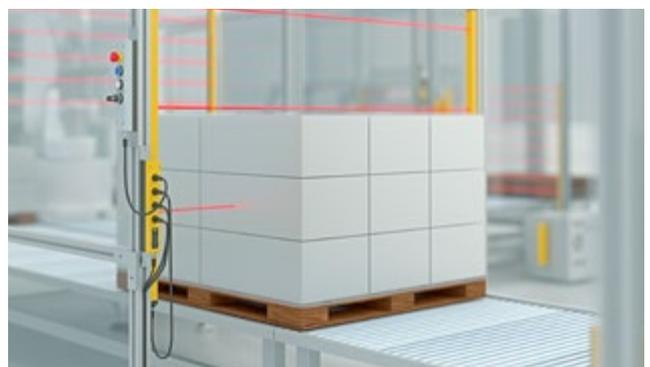
For the safe unloading of complex pallets or small components, the SSP ready-to-use interlocking function can be used.
