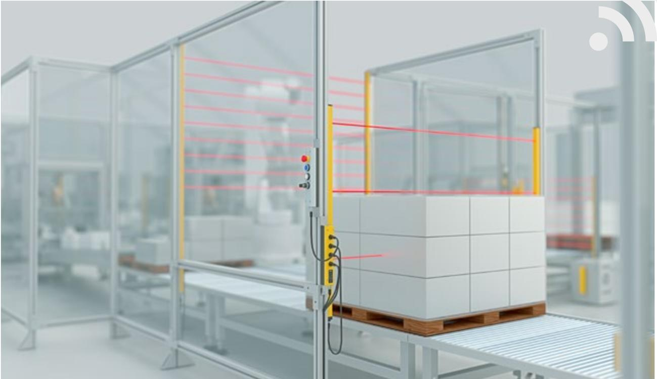
Safety Simplifier interlocking function with EOS4 light grids for unloading of pallets
