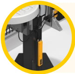
At the tool stand, the Safety Simplifier monitors the safe tool change of the robot.
