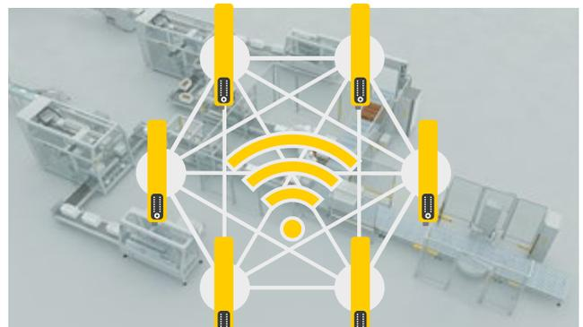
Using a wireless mesh network, the Safety Simplifier ensures that your safety signals reach their destination reliably and safely by the fastest route.
