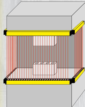
Safe guarding of a C press on 3 sides without obstruction through vertical tilted mirror.
