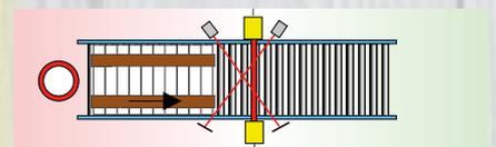
Muting variation cross-muting. The intersection point of both light barrier beams must be within the danger zone.
