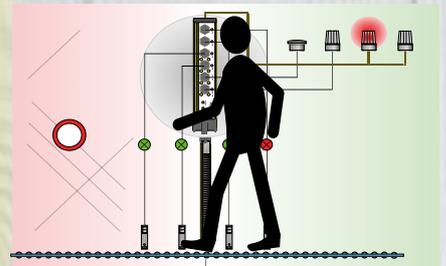
If the light barriers are arranged correctly, people will not simultaneously interrupt the muting light barrier pairs A or B.
