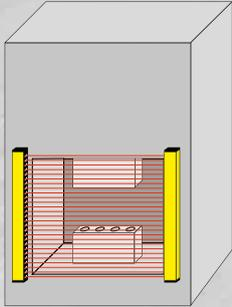
Multi-beam safety light curtains for safeguarding off hazardous areas. Finger or hand protection.
