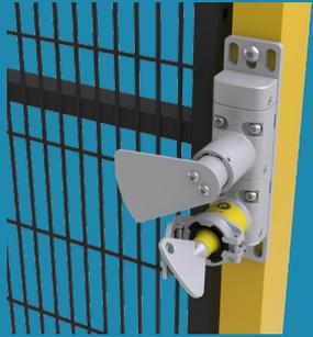
When the safety contacts of the existing system are opened the 'Door Blocking Plate' prevents the door opening until key is removed
