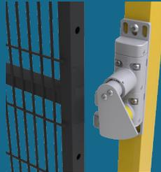
The door blocking plate is sprung to allow the door to open
