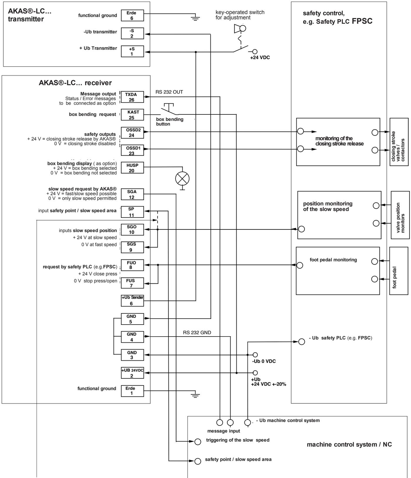
**Bridge SP - SGO / SGS:** only if the machine control does not indicate any safety point or slow speed range. Short strikes within the slow speed range by activating the footpedal twice are only possible, if the valves are not yet in the slow speed position at the start of the stroke, but if the AKAS® light beams have been interrupted before.
