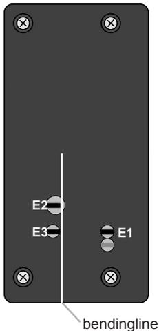
view after removing the connection lid on the receiver
