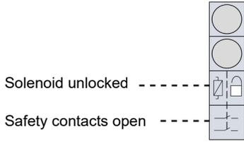
Access keys unlocked, safety contacts open.
