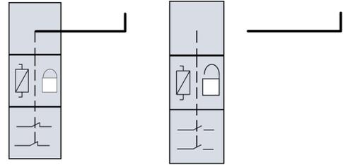
Guard is locked until machine stops, guard unlocking opens safety switches
