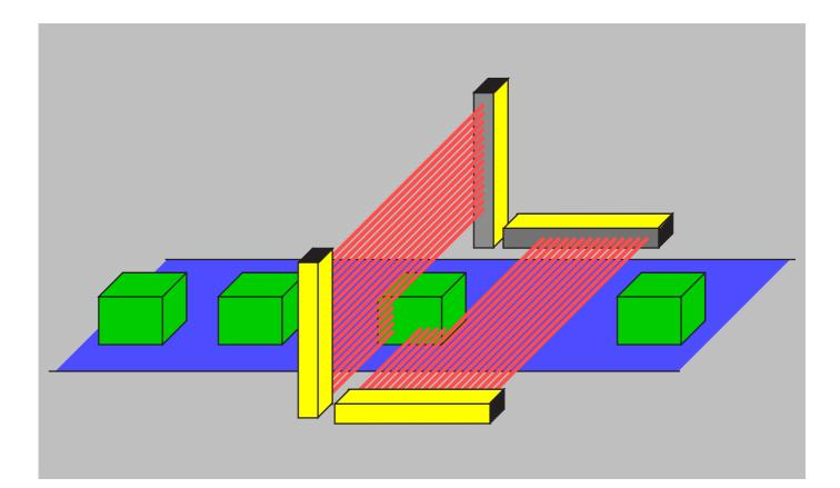
Parallel scanning - therefore no error of measurement
