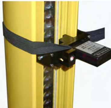
Column mounting mount the elastic band only on one screw
