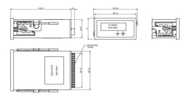
Rail Housing Terminals Weight Rail DIN 46277-3 (EN 50022) or mounting plate to DIN 43660 (41612)
